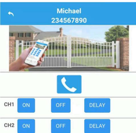
**CALL:** click this "CALL" icon button to turn on/off CH1 relay or activate CH1/CH2 related working mode fast
